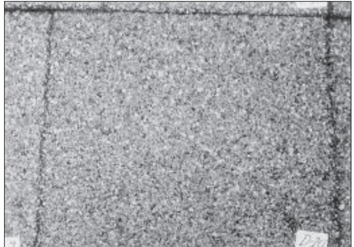
Photo D2. Close-up of D-10 before impacting at 10 years 6 months weathering exposure.
