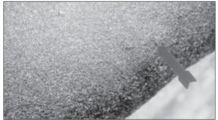
Photo 5. Close-up on bottom side of D-7 of half-panel designation CO-TS-D-7 at impact site. Note single-line fracture pattern weathered 4 years 4 months.
